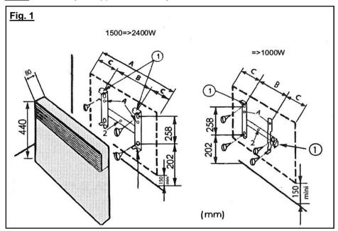
The heater must not be located immediately below a socket outlet (as per requirement of Clause 7.12 of AS/NZS 60335.2.30).
